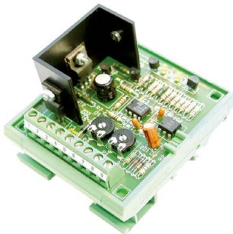
**Slope separation:** To avoid simultaneous clutch and braking torques, a slope separation of 0 – 100 ms between clutch and brake can be set, which acts according to the respective attraction time and drop-out time of the coils (see switching time table). This adjustment is carried out via the potentiometers Ku = clutch (P2) and Br = brake (P1). The factory default setting is 0 ms.
