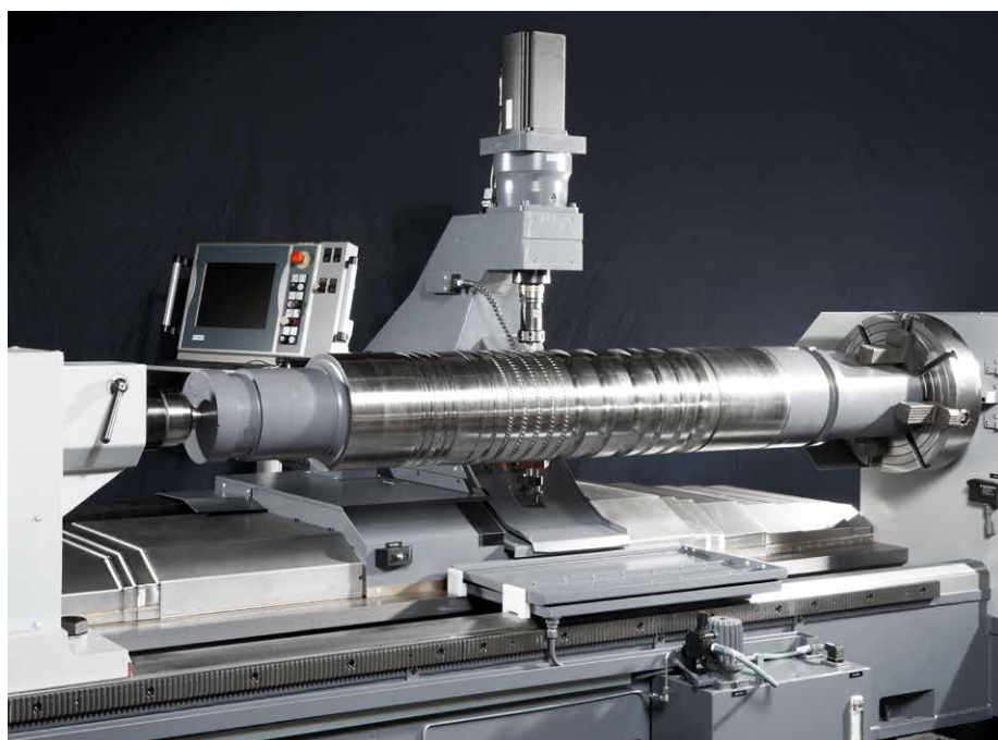
Gearbox ES-1247 serving as a spindle drive of a notch milling machine NNF made by Herkules
