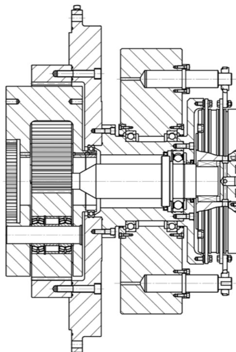
Clutch-brake with planetary gear.
