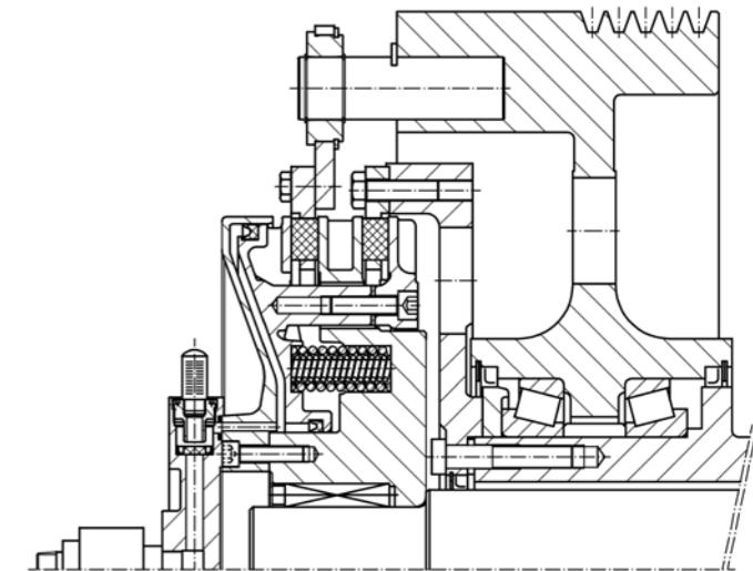
Clutch-brake unit with quick exhaust. To get very quick braking response time.
