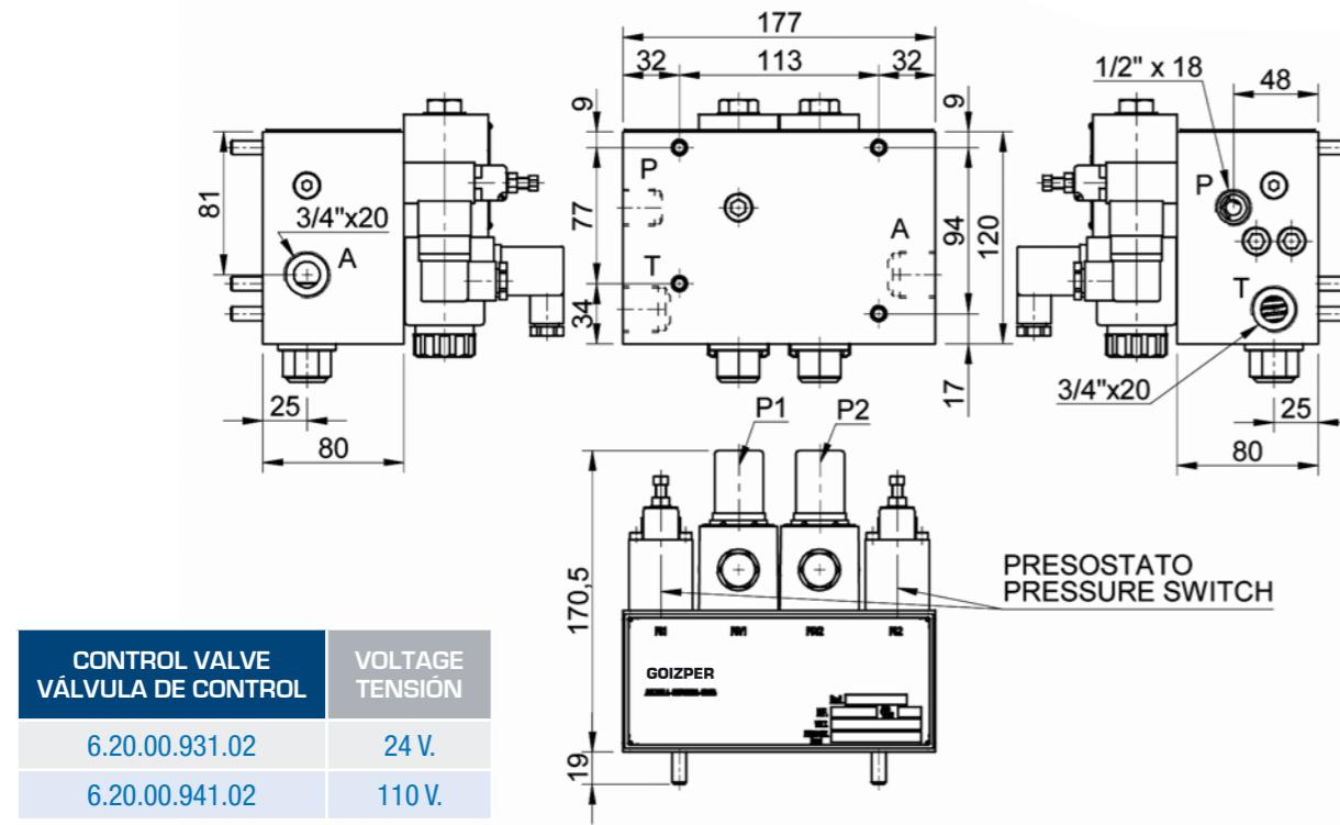
The press safety valve (2EV) is mainly used to control the hydraulically actuated conventional combined clutch-brakes.
