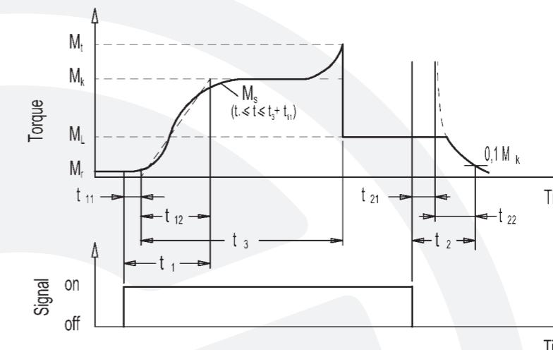
**Slip or dynamic torque  $M_s$ :** this is the torque transmitted once the torque increase time ( $t_{12}$ ) is finished. It changes within the cycle process and depends, apart from other factors, on the slip speed and the temperature of the friction surfaces.
