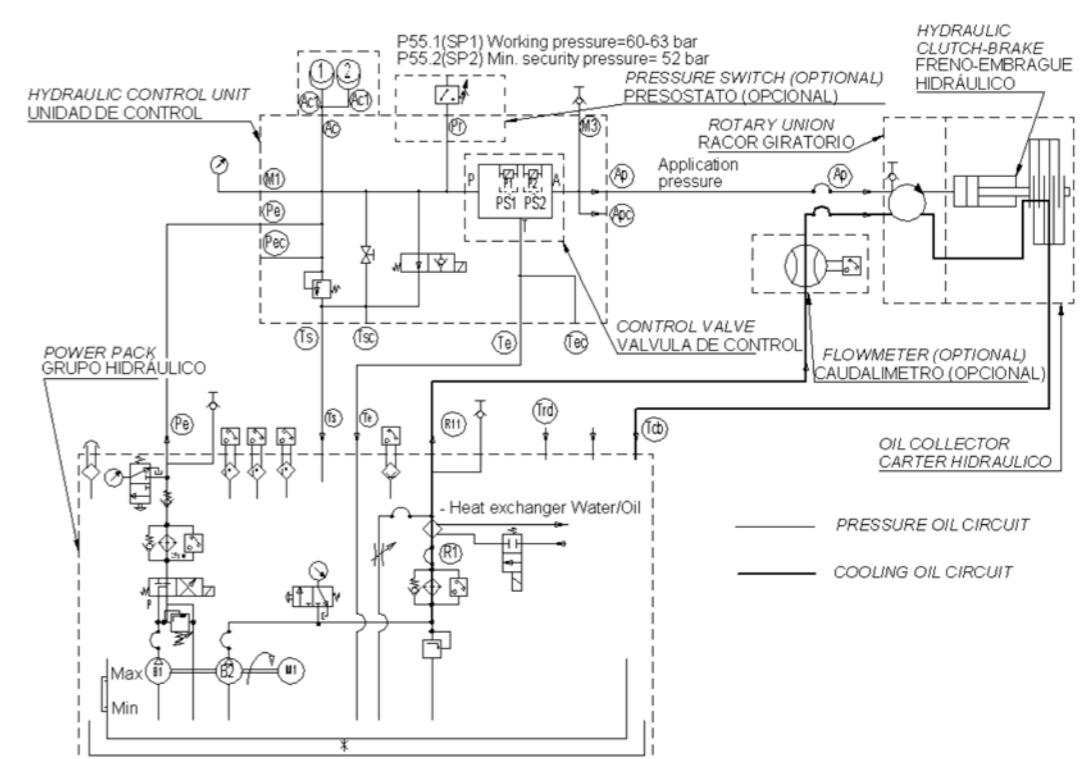
In order to size the equipment properly, according with the operating data provided by the customer, GOIZPER will indicate the oil flow rates required for each circuit and the required accumulator and heat exchanger capacities.
