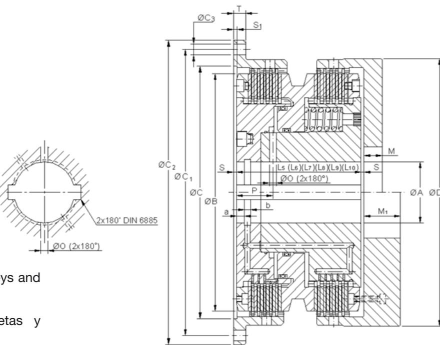
Mounting on the shaft by keys and oil inlet through the shaft.
