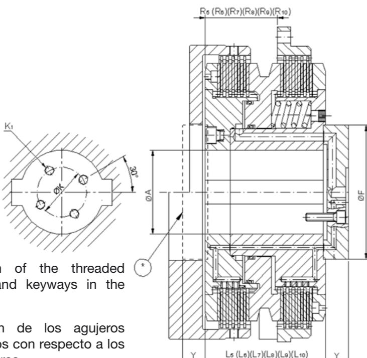
Mounting on the shaft by keys and oil inlet through the hub.
