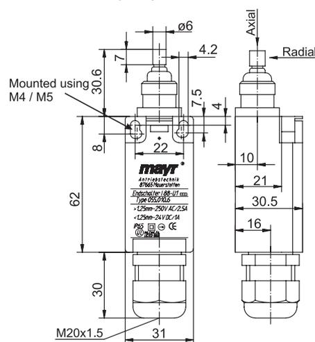
Fixed positioning for safety application with fixing screws 2 x M5 (DIN 921).
