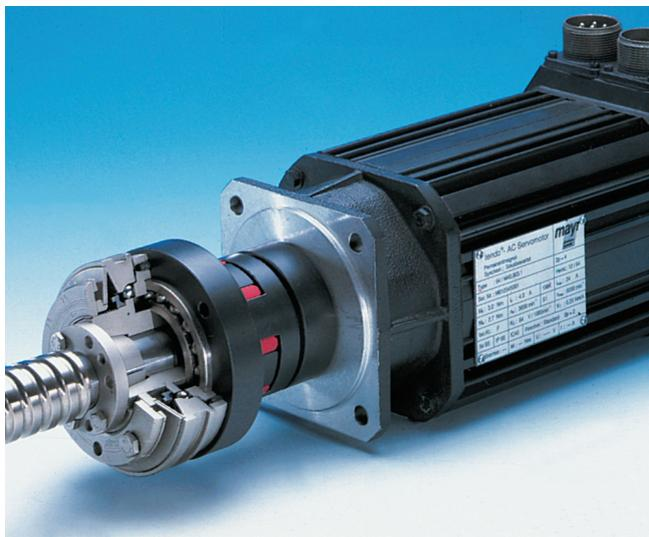
EAS<sup>®</sup>-NC Lastic Backlash-free version in a directly driven servo axis. This combination limits the torque precisely to the pre-set value, compensates for shaft misalignments and damps critical vibrations.
