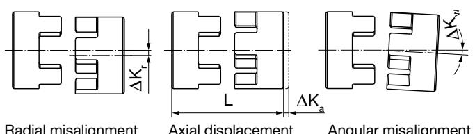
Radial misalignment      Axial displacement      Angular misalignment
