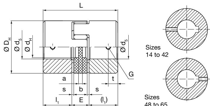
The adjusting screw is offset by 180° to the keyway on Sizes 14 to 42 (see Fig. above).
