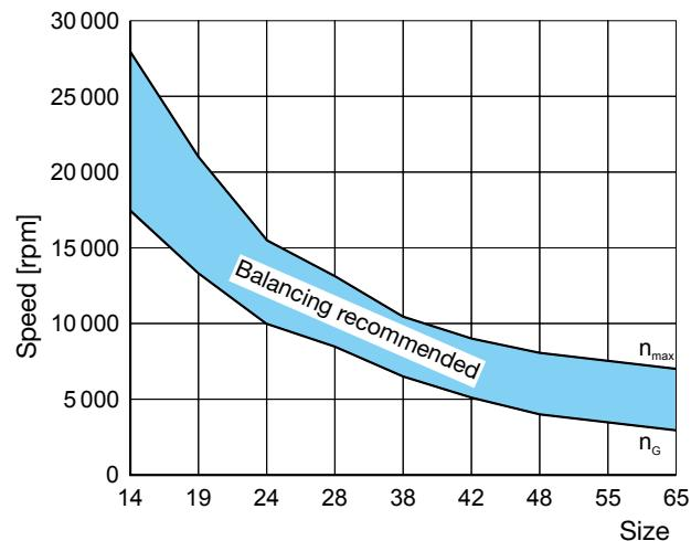
Diagram 1: Balancing the Shrink Disk Hubs
