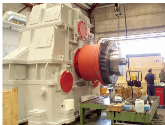
Jaure MTGX-HD-TI-1000 on wind test bench
