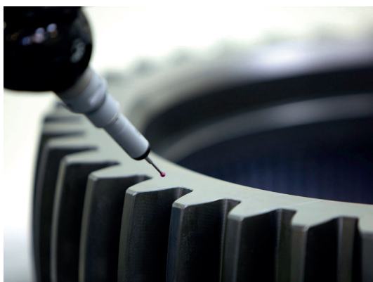
Gear inspection in CMM
