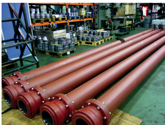
Jaure gear coupling for underwater operation
